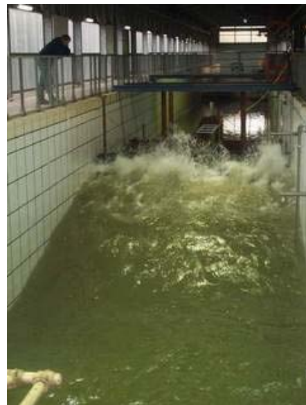
Fig. 4. Testing of the breakwater using an irregular wave train (JONSWAP spectrum) in the GWK.
