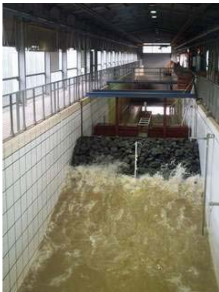
Fig. 4. Testing of the breakwater using an irregular wave train (JONSWAP spectrum) in the GWK.
