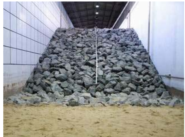
Fig. 3. The run-up gauge (designed and constructed at Ghent University) mounted on the seaward (1:2) slope of the breakwater.
