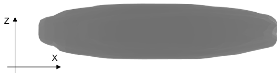
Figure 4 3D STL volume of a defect obtained from 3D NDE.
